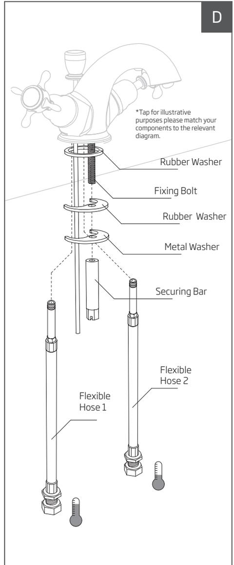
5. Fit the mixer body to the basin / bidet using the supplied rubber washer, metal washer and fixing nut in the order indicated in the drawings A to D.
